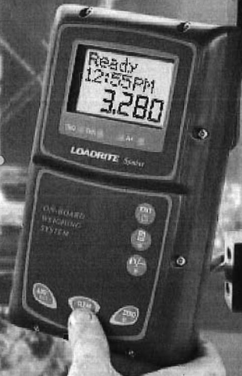
Install the LOADRITE® Sprint™ on your forklift or small wheel loader and see how you'll save time and money. This cost-effective onboard weighing system combines basic functions required to load once and load right, along with the exceptional service and support that LOADRITE® provides. With only six keys the LOADRITE® Sprint™ is operator friendly and simple to use.
